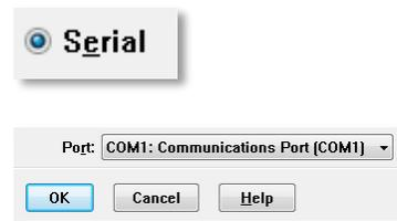
6. Connection: If using Tera Term, the emulator should start logging data from the BACTROX-2 once every minute if the correct com port was chosen. If the emulator is not logging the data, perform the following steps.
