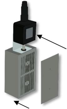
4. Attach the calibration gas sample to the O<sub>2</sub> CAL PORT.
