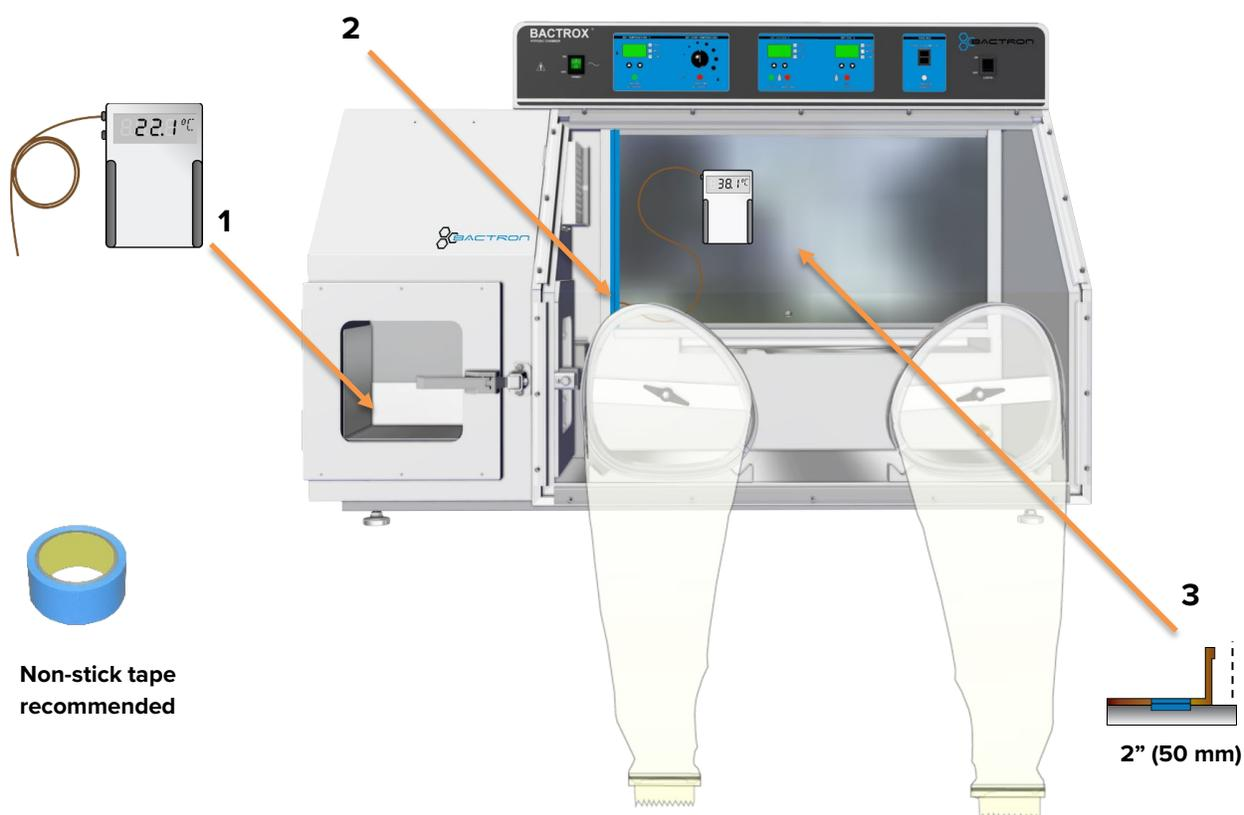
3. Position the thermocouple probe head as near as possible to the geometric center of the chamber. The head be at least 2 inches (50 mm) from the shelf surface to prevent heatsinking. Secure the thermocouple probe to the shelving with non-marking tape.
