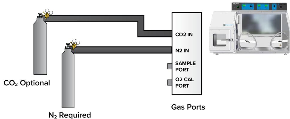
Match the correct gas regulator type to the correct gas type. A CO<sub>2</sub> regulator should always be used for CO<sub>2</sub> supplies, etc.
