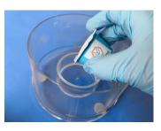
3. Prime wick for 60 seconds in reagent reservoir of MycoFog<sup>™</sup>
